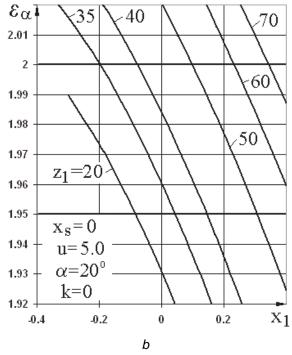
Fig. 5.  $\varepsilon_{\alpha}$ =f(x<sub>1</sub>, , z<sub>1</sub> u=2, $\alpha$ =20°, x<sub>s</sub>=0, k=0)
