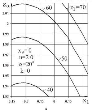
is obtained also at smaller teeth numbers of pinion  $(z_1 \ge 30)$ .
